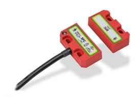
IDEM safety switch set, non-contact coded magnetic, (2) N.C. safety output(s), (1) N.O. monitoring output(s), plastic housing, 50 x 25mm, pigtail, 16.4ft/5m cable length.
