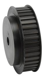
SureMotion timing pulley, steel, 3/8in L pitch, 40 tooth, 4.775in pitch diameter, 5/8in bore, hub with flanges. For use with 1in wide belt.
