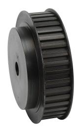
SureMotion timing pulley, steel, 3/8in L pitch, 40 tooth, 4.775in pitch diameter, 5/8in bore, hub with flanges. For use with 1in wide belt.
