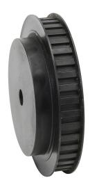
SureMotion timing pulley, steel, 3/8in L pitch, 40 tooth, 4.775in pitch diameter, 1/2in bore, hub with flanges. For use with 1/2in wide belt.
