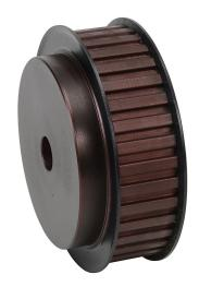
SureMotion timing pulley, steel, 3/8in L pitch, 36 tooth, 4.297in pitch diameter, 5/8in bore, hub with flanges. For use with 1in wide belt.
