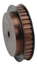
SureMotion timing pulley, steel, 3/8in L pitch, 36 tooth, 4.297in pitch diameter, 1/2in bore, hub with flanges. For use with 1/2in wide belt.
