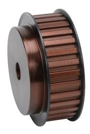
SureMotion timing pulley, steel, 3/8in L pitch, 32 tooth, 3.82in pitch diameter, 5/8in bore, hub with flanges. For use with 1in wide belt.
