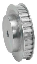
SureMotion timing pulley, steel, 3/8in L pitch, 32 tooth, 3.82in pitch diameter, 1/2in bore, hub with flanges. For use with 1/2in wide belt.
