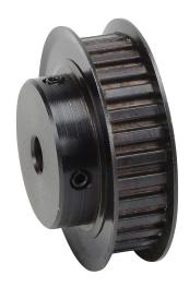
SureMotion timing pulley, steel, 1/5in XL pitch, 30 tooth, 1.91in pitch diameter, 5/16in bore, hub with flanges. For use with 3/8in wide belt.
