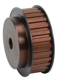
SureMotion timing pulley, steel, 3/8in L pitch, 30 tooth, 3.581in pitch diameter, 5/8in bore, hub with flanges. For use with 1in wide belt.
