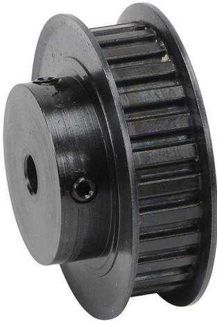
SureMotion timing pulley, steel, 1/5in XL pitch, 28 tooth, 1.783in pitch diameter, 1/4in bore, hub with flanges. For use with 3/8in wide belt.
