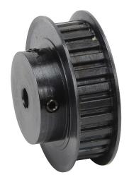
SureMotion timing pulley, steel, 1/5in XL pitch, 28 tooth, 1.783in pitch diameter, 1/4in bore, hub with flanges. For use with 3/8in wide belt.
