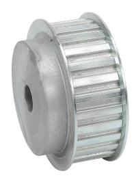
SureMotion timing pulley, steel, 3/8in L pitch, 28 tooth, 3.342in pitch diameter, 5/8in bore, hub with flanges. For use with 1in wide belt.
