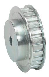
SureMotion timing pulley, steel, 3/8in L pitch, 28 tooth, 3.342in pitch diameter, 1/2in bore, hub with flanges. For use with 1/2in wide belt.
