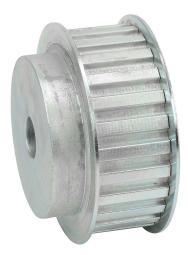
SureMotion timing pulley, steel, 3/8in L pitch, 26 tooth, 3.104in pitch diameter, 5/8in bore, hub with flanges. For use with 1in wide belt.
