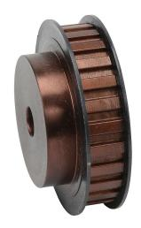
SureMotion timing pulley, steel, 3/8in L pitch, 26 tooth, 3.104in pitch diameter, 1/2in bore, hub with flanges. For use with 1/2in wide belt.
