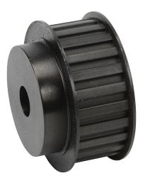
SureMotion timing pulley, steel, 3/8in L pitch, 24 tooth, 2.865in pitch diameter, 5/8in bore, hub with flanges. For use with 1in wide belt.
