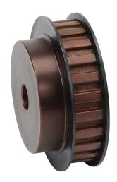
SureMotion timing pulley, steel, 3/8in L pitch, 24 tooth, 2.865in pitch diameter, 1/2in bore, hub with flanges. For use with 1/2in wide belt.
