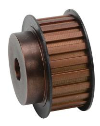
SureMotion timing pulley, steel, 3/8in L pitch, 22 tooth, 2.626in pitch diameter, 5/8in bore, hub with flanges. For use with 1in wide belt.
