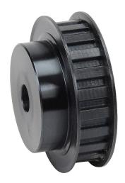
SureMotion timing pulley, steel, 3/8in L pitch, 22 tooth, 2.626in pitch diameter, 1/2in bore, hub with flanges. For use with 1/2in wide belt.
