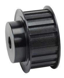
SureMotion timing pulley, steel, 3/8in L pitch, 20 tooth, 2.387in pitch diameter, 1/2in bore, hub with flanges. For use with 1in wide belt.
