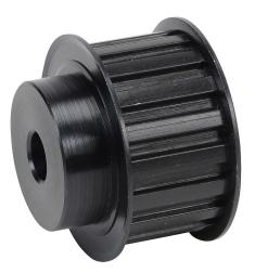
SureMotion timing pulley, steel, 3/8in L pitch, 18 tooth, 2.149in pitch diameter, 1/2in bore, hub with flanges. For use with 1in wide belt.
