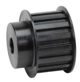
SureMotion timing pulley, steel, 3/8in L pitch, 16 tooth, 1.91in pitch diameter, 1/2in bore, hub with flanges. For use with 1in wide belt.
