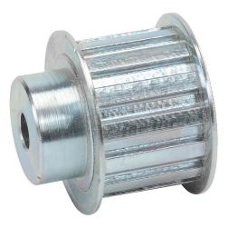
SureMotion timing pulley, steel, 3/8in L pitch, 14 tooth, 1.671in pitch diameter, 3/8in bore, hub with flanges. For use with 1in wide belt.
