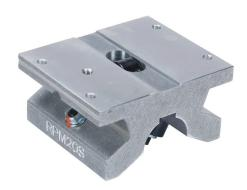
PBC SPB series single roller pillow block, cam follower bearing, 3.37in overall length, steel, 1-1/4in inside diameter, aluminum housing, adjustable running clearance. For use with 1-1/4in diameter PBC shafts.
