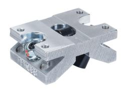
PBC SPB series single roller pillow block, cam follower bearing, 1.5in overall length, steel, 1/2in inside diameter, aluminum housing, adjustable running clearance. For use with 1/2in diameter PBC shafts.
