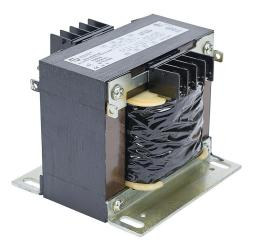
Hammond control transformer, open core, 750 VA, 1-phase, 208/416 VAC primary, 120/240 VAC secondary, 50/60 Hz, panel mount.
