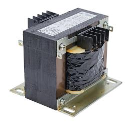
Hammond control transformer, open core, 750 VA, 1-phase, 240/480 VAC primary, 120/240 VAC secondary, 50/60 Hz, panel mount.
