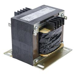
Hammond control transformer, open core, 750 VA, 1-phase, 480/600 VAC primary, 120/240 VAC secondary, 60 Hz, panel mount.
