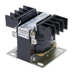
Hammond control transformer, open core, 50 VA, 1-phase, 240/480 VAC primary, 120/240 VAC secondary, 50/60 Hz, panel mount.
