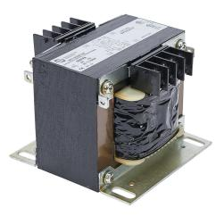
Hammond control transformer, open core, 500 VA, 1-phase, 480/600 VAC primary, 120/240 VAC secondary, 60 Hz, panel mount.
