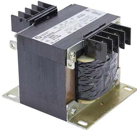
Hammond control transformer, open core, 350 VA, 1-phase, 208/416 VAC primary, 120/240 VAC secondary, 50/60 Hz, panel mount.
