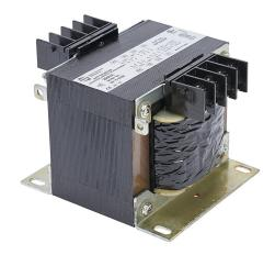
Hammond control transformer, open core, 350 VA, 1-phase, 208/416 VAC primary, 120/240 VAC secondary, 50/60 Hz, panel mount.
