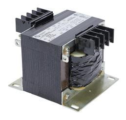
Hammond control transformer, open core, 350 VA, 1-phase, 240/480 VAC primary, 120/240 VAC secondary, 50/60 Hz, panel mount.
