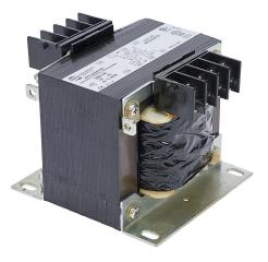
Hammond control transformer, open core, 350 VA, 1-phase, 480/600 VAC primary, 120/240 VAC secondary, 60 Hz, panel mount.
