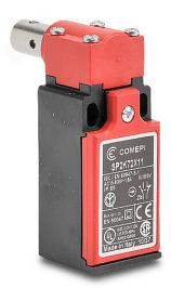
Comepi safety switch, hollow shaft hinge interlock, slow action break before make, (1) N.C. safety output(s), plastic body, plastic head, 12mm diameter x 20mm length shaft, (1) PG11 cable entry with 1/2in NPT adapter.
