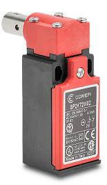
Comepi safety switch, hollow shaft hinge interlock, slow action, (2) N.C. safety output(s), plastic body, plastic head, 12mm diameter x 20mm length shaft, (1) PG11 cable entry with 1/2in NPT adapter.
