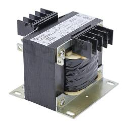
Hammond control transformer, open core, 250 VA, 1-phase, 208/416 VAC primary, 120/240 VAC secondary, 50/60 Hz, panel mount.
