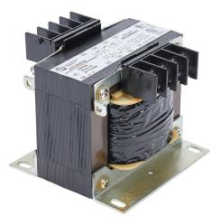
Hammond control transformer, open core, 250 VA, 1-phase, 240/480 VAC primary, 120/240 VAC secondary, 50/60 Hz, panel mount.
