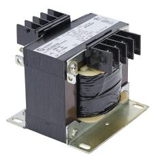
Hammond control transformer, open core, 250 VA, 1-phase, 480/600 VAC primary, 120/240 VAC secondary, 60 Hz, panel mount.
