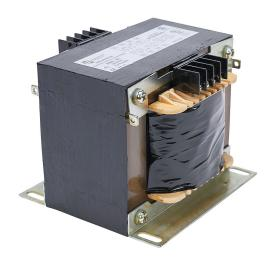
Hammond control transformer, open core, 2 kVA, 1-phase, 240/480 VAC primary, 120/240 VAC secondary, 50/60 Hz, panel mount.
