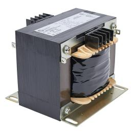
Hammond control transformer, open core, 2 kVA, 1-phase, 480/600 VAC primary, 120/240 VAC secondary, 60 Hz, panel mount.
