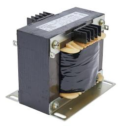
Hammond control transformer, open core, 1.5 kVA, 1-phase, 208/416 VAC primary, 120/240 VAC secondary, 50/60 Hz, panel mount.
