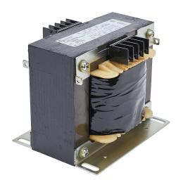
Hammond control transformer, open core, 1.5 kVA, 1-phase, 208/416 VAC primary, 120/240 VAC secondary, 50/60 Hz, panel mount.
