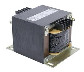
Hammond control transformer, open core, 1.5 kVA, 1-phase, 480/600 VAC primary, 120/240 VAC secondary, 60 Hz, panel mount.
