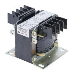
Hammond control transformer, open core, 100 VA, 1-phase, 480/600 VAC primary, 120/240 VAC secondary, 60 Hz, panel mount.
