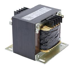
Hammond control transformer, open core, 1 kVA, 1-phase, 208/416 VAC primary, 120/240 VAC secondary, 50/60 Hz, panel mount.
