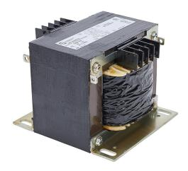
Hammond control transformer, open core, 1 kVA, 1-phase, 480/600 VAC primary, 120/240 VAC secondary, 60 Hz, panel mount.
