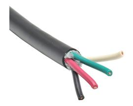
Direct Wire portable cord, unshielded, SOOW, 600V, 4 conductors (includes ground), 8 AWG, EPDM thermoset rubber conductor insulation material, black, white, red and green, CPE thermoset rubber jacket, black, cut to length.
