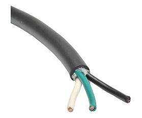
Direct Wire portable cord, unshielded, SOOW, 600V, 3 conductors (includes ground), 8 AWG, EPDM thermoset rubber conductor insulation material, black, white and green, CPE thermoset rubber jacket, black, cut to length.
