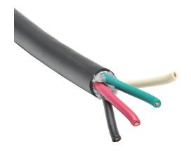
Direct Wire portable cord, unshielded, SOOW, 600V, 4 conductors (includes ground), 6 AWG, EPDM thermoset rubber conductor insulation material, black, white, red and green, CPE thermoset rubber jacket, black, cut to length.
