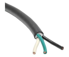
Direct Wire portable cord, unshielded, SOOW, 600V, 3 conductors (includes ground), 6 AWG, EPDM thermoset rubber conductor insulation material, black, white and green, CPE thermoset rubber jacket, black, cut to length.
