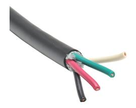
Southwire portable cord, unshielded, SOOW, 600V, 4 conductors (includes ground), 18 AWG, EPDM thermoset rubber conductor insulation material, black, white, red and green, CPE thermoset rubber jacket, black, cut to length.
