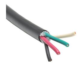
Southwire portable cord, unshielded, SOOW, 600V, 4 conductors (includes ground), 18 AWG, EPDM thermoset rubber conductor insulation material, black, white, red and green, CPE thermoset rubber jacket, black, cut to length.
