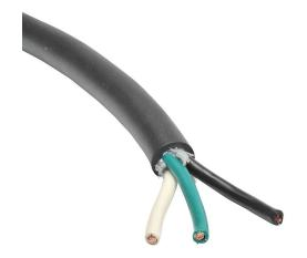
Southwire portable cord, unshielded, SOOW, 600V, 3 conductors (includes ground), 18 AWG, EPDM thermoset rubber conductor insulation material, black, white and green, CPE thermoset rubber jacket, black, cut to length.
